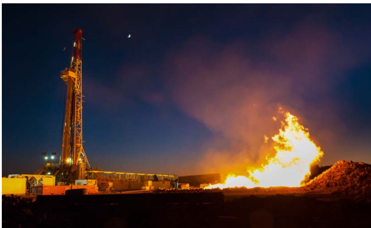
Figure 4: PV13 Flow test from the Pacoota Sandstone, approximately 13 mcf per day (13TJ/day)
