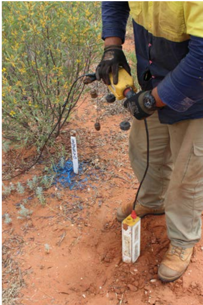
Figure 3: Geophone array placement to receive reflected acoustic signal.
