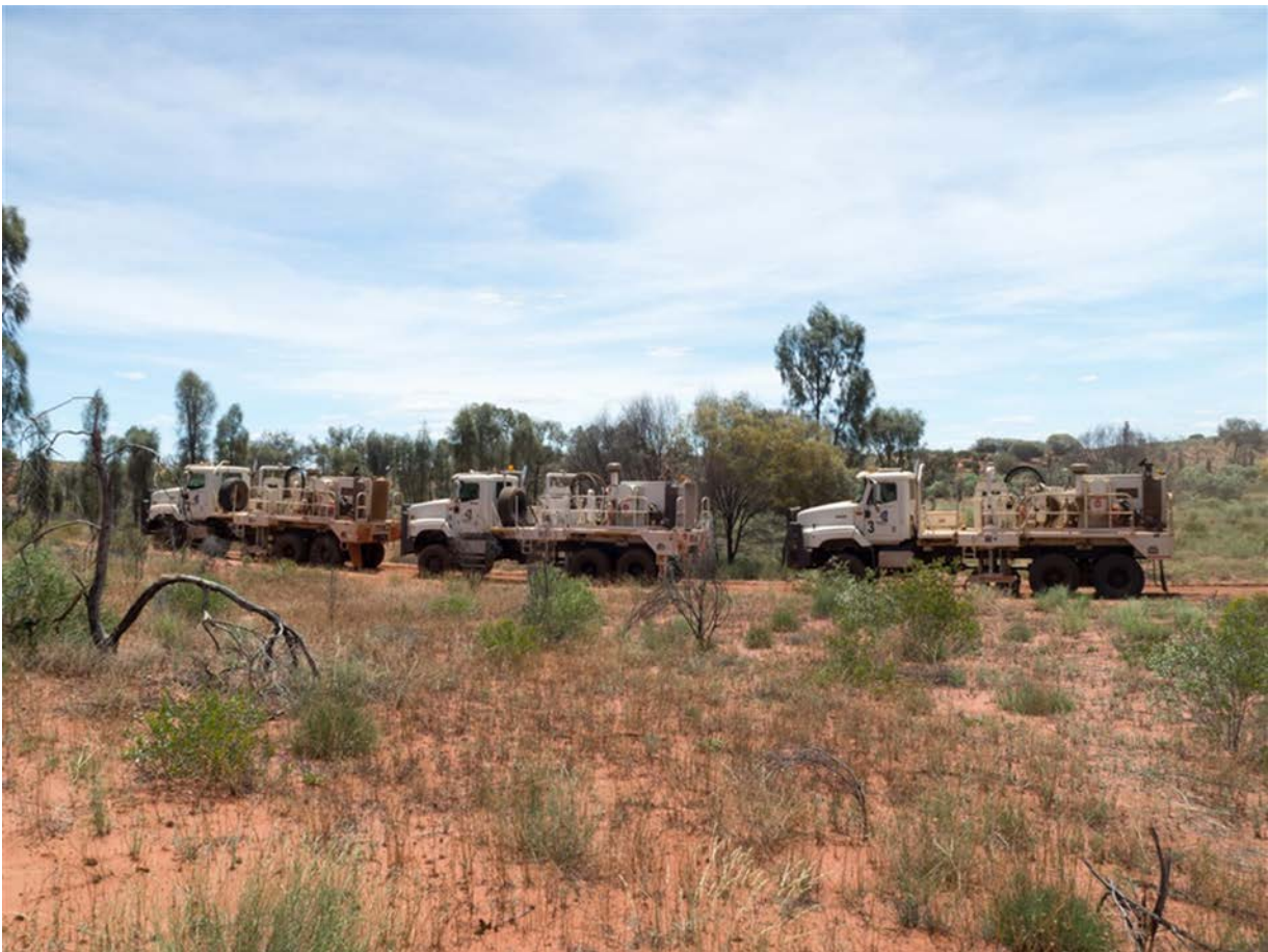
Figure 2: Seismic vibrator array providing energy to image sub-surface horizons.
