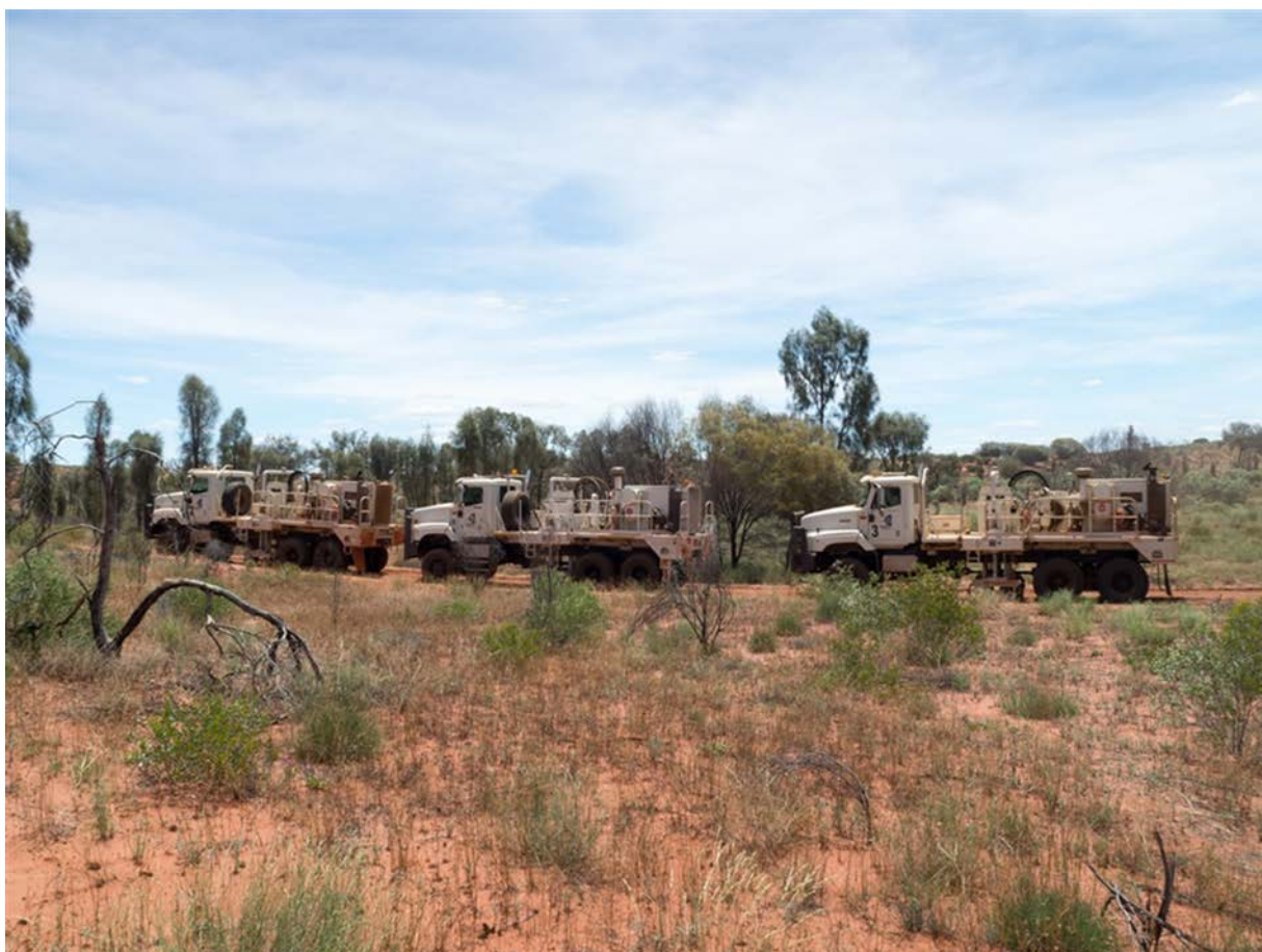
Figure 1: Seismic vibrator array providing energy to image sub-surface horizons.
